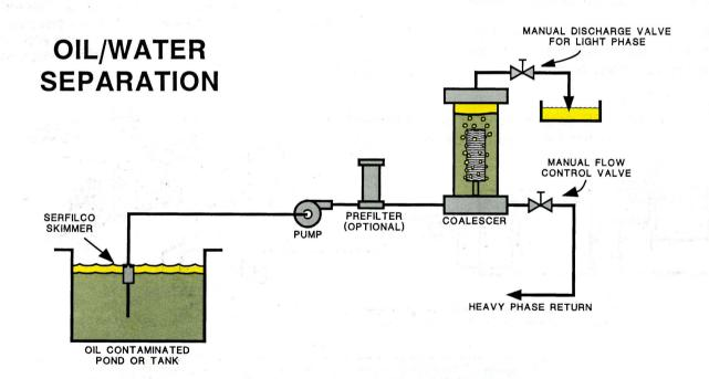
The coalescing element normally is not replaced and has an indefinite life. It needs replacement only in the event that it becomes plugged with solid particles. Therefore, if the unit is to be used in a system that has solids contamination, a pre-filter is recommended. The individual components of the system feature non-metallic solution contact for use with corrosive liquids. Consult factory to obtain information on larger or specially designed systems.
