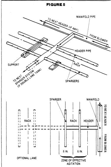
blower system layout. Note the elbow or loop arrangement of the air delivery piping, including an antisiphon hole above the liquid level of the tank to avoid ingestion of solution by the blower at the moment the air system is turned off. A check valve may also be used if desired.
