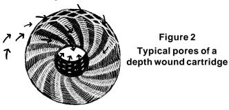
Cleaners require 50 to 75 micron. Hexavalent chrome will use 30 to 50 micron on most baths but some work may require 15. Trivalent chrome uses 1 to 5 micron. Copper and nickel are typically filtered to 15 micron.
