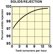
Hydraulics indicate a turnover rate of 14 times is required to have all the liquid pass through the filter once.
