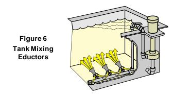
Tank Mixing Eductors have provided a new solution to these problems. The TME is a special designed thermoplastic device which, when placed in a tank at the discharge of a pump or filter system, will deliver 5 GPM (19.4 l/min) of flow for every 1 GPM (3.8 l/min) fed to it.
