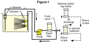
A typical sequence would be to agitate and high flow filter during working hours. At night, without agitation, liquid would pass through filter and optional coalescer at low flow to remove oils.
