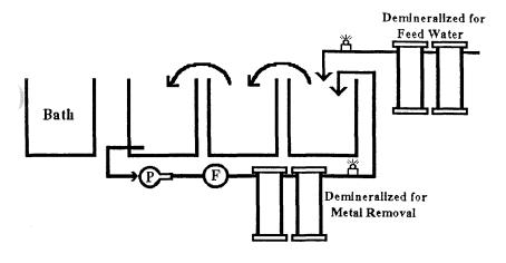
By closing the loop, you can achieve zero discharge. The make up water is deionized to decrease the load of solids on the second metal removal deionizer. Also, by deionizing your make up water, your product will be cleaner and spot free. The second deionizer removes the metals, and recirculates the water through the rinse baths. Each deionizer is equipped with a water quality light to help you determine when to exchange the resin pack.
