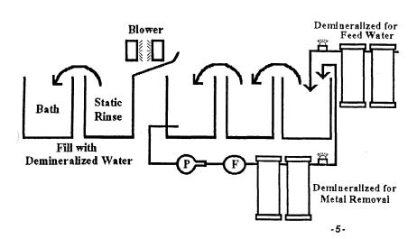
A static rinse can be installed between the plating bath and rinse tanks. In addition, a car wash type blower can be installed to remove drag out and blow it back into the static rinse tank. This has two benefits: 1) it reduces the load on the rinse tanks (and thus on the metal removal packs), and 2) in many cases, it's a valuable resource for make up to the plating bath. The water that makes up the static rinse should be deionized.
