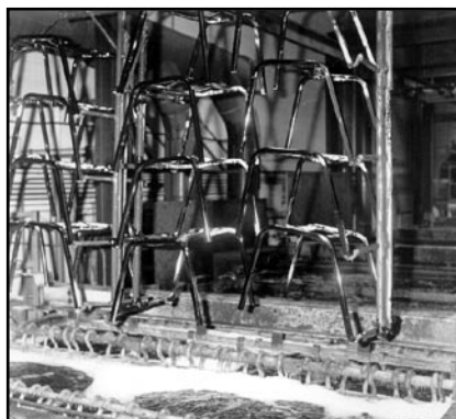
Tubular work over nickel plating tank.
