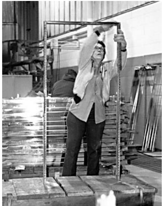
Final inspection is done by an operator wearing gloves to help detect roughness. Better cleaning and improved filtration have reduced roughness and lowered reject rates.
