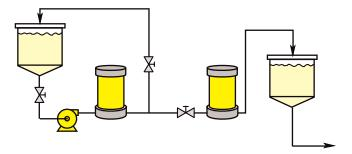
solids holding capacity offered by coarser media. Coarse media may provide up to five times the solids retention before flow is reduced to an unacceptable rate, or if monitored, recirculation may be used until a desired clarity is achieved, at which time the valves (see diagram) are moved to direct the clean liquid to the clean storage tank. Additional recirculation of the clean tank may also be done and a second trap filter using denser media may also be used. (See diagram)
