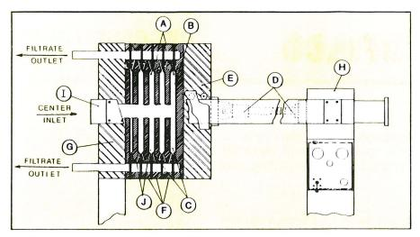
Dewatering is accomplished by pumping a slurry or sludge into chambers (A) surrounded by filter membranes (B). As pumping pressure is increased the filtrate is forced through the accumulated filter cake (C) and membrane until the chamber is full of solid filter cake.
