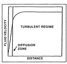
notional thickness which can be described by the concentration gradients of the active species and is a function of viscosity, temperature, density and velocity. The thickness of this layer frequently determines the rate of chemical or electrochemical reaction, i.e. the deposition rate. Thus, we have the limiting current density rate at which the speed of plating is restricted by the speed at which the metal ions being deposited can be replaced by fresh ions moving through the barrier layer.
