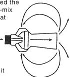
How does the eductor concept work? An eductor is simply a venturi from which the reducing and throat sections have been removed. In their place is an orifice nozzle, as shown in the simplified diagram above.
