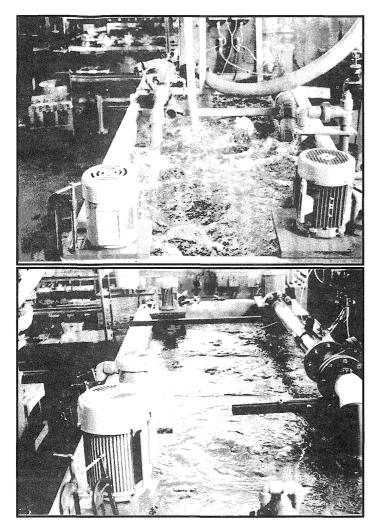
**AIR AGITATED SOLUTION** with bubbles exploding at the surface, often creating an unwanted mist, as typically found in plating, cleaning and/or waste treatment.
