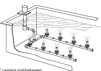
Note that eductors are on 24" centers and between them are threaded, plugged holes. If a more thorough pattern of agitation is desired, remove plugs and replace with eductors. Eductors can be rotated 360° to change direction of solution flow.
