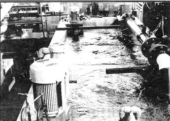
AIR AGITATED SOLUTION with bubbles exploding at the surface, often creating an unwanted mist, as typically found in plating, cleaning and/or waste treatment.
