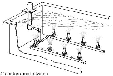
Note that eductors are on 24" centers and between them are threaded, plugged holes. If a more thorough pattern of agitation is desired, remove plugs and replace with eductors. Eductors can be rotated 360° to change direction of solution flow.
