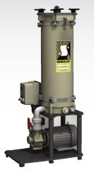
You need a **FILTER** to remove the soils you loosened from the parts in the soak cleaner
