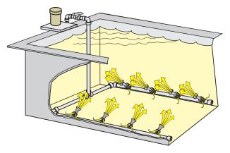
**BUT...** how will I be able to plate fast without the agitation needed to transfer the ions from the anodes or solution to my parts . . . the answer is – **change** over to pumped agitation (Ser-Ducting®) using the natural phenomenon of a venturi which will multiply your pump flow capacity five-fold. This now can provide 50-100 turnovers per minute
