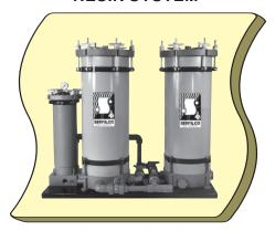
Recover heavy metals from rinse water. Effluent is suitable for discharge or bath replenishment. Concentrated regenerate can be chemically treated for disposal or possible recovery. Choice of systems with or without prefilters (prefilter removes suspended solids that decrease resin capacity). Flow rates to 480 GPH.
