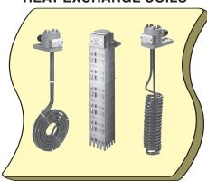
For heating or cooling cleaners, plating baths and virtually all acids and alkalies. Safeguard protector cuts off power in over-temperature conditions. Available in over-the-side, L-shaped or side entry. Quartz, stainless steel, titanium or TFE.
