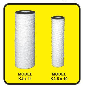
These high efficiency coalescing elements are designed to reduce the level of the separated liquid - oil, water, etc. - to 10 ppm or less. This high efficiency is attributable to the manufacturing process that produces a precise fiber pattern with progressively larger openings in the direction of fluid flow. This design maximizes the coalescing process by permitting the oil, water or other contaminating liquid to unite and form a distinctly separate and removable fluid.
