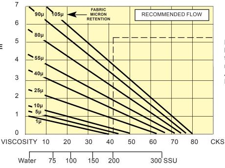
NOTE: Confirm data beyond 200 SSU by testing fluid with fabric media. Contact Application Engineering Dept. for sample fabric.
