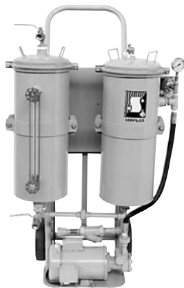
Portable filter system equipped with a large capacity filter chamber for removing solid contaminants from hydraulic oil and a coalescing chamber for removing water. Unit can be wheeled from machine to machine, as needed.
