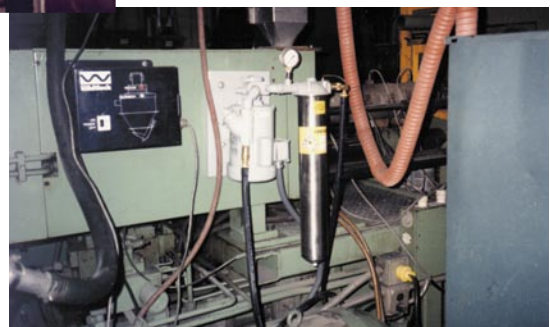
Portable filter system equipped with a large capacity filter chamber for removing solid contaminants from hydraulic oil and a coalescing chamber for removing water. Unit can be wheeled from machine to machine, as needed.
