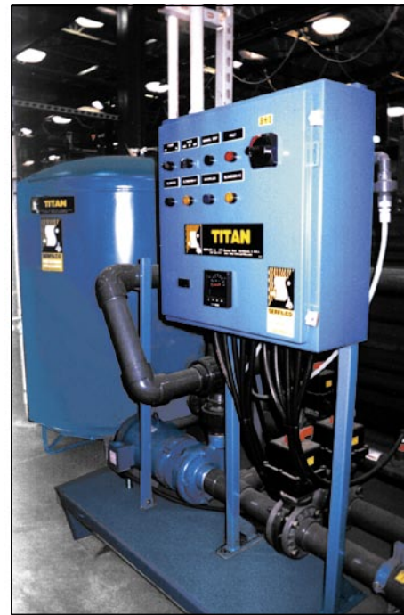
IEP's TITAN filter system showing control panel and piping in foreground and filter chamber in the background.
