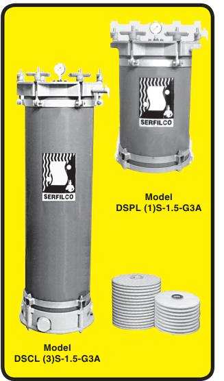
**SERIES 'DS' Filter chambers** are designed to accommodate combinations of 1 to 4 9-disc or 1 to 3 16-disc Disc-Sets by use of spacer spools which are included with each assembly. Design features top access for quick and easy Disc-Set removal and replacement while shell remains sealed to base. Capability of a single chamber to accommodate Disc-Set combinations significantly reduces operating cost and downtime. On-site selection of 180° or 90° entry to exit is an added piping convenience.
