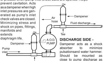
possible to absorb shock at its source. Will prevent leaking joints and fittings due to pulsation. Allows meters to be used without damage and extends the life and reliability of pump components.
