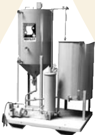
OIL RECONDITIONING STATION for salvaging oils in large volume
