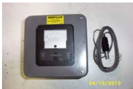
Conductivity Monitor; Corrosion resistant NEMA 3 enclosure; 115 vac,50-60 Hz Comment: 0-500 micromhos conductivity measurements
